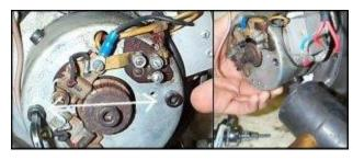
3. Use the 5mm allen wrench (supplied in the kit) and remove the two socket head cap screws which retain the field of the generator to the front timing gear cover of the engine. Gently remove the field from the gear cover and set it aside. It is sometimes necessary to gently bump the side of the generator field with a mallet to dislodge it from the cover.
