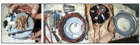
5. Remove the four 5mm socket head cap screws from the face of the stator with a 4mm allen wrench supplied in the kit. Disassemble the stator housing of the alternator and separate the back housing from the windings. Remove the back cover of the stator. Remove and discard the paper wrapping from the rotor.
