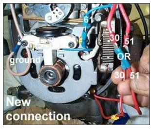
screws, on the face of the alternator and install the ring terminal of the brown wire under the head of the socket head cap screw. Re-tighten the cap screw.
